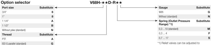
\*1) Relief valves can be adjusted to pressures in excess of, and less than, those specified. Do not use these units to control pressures outside of the specified ranges.
